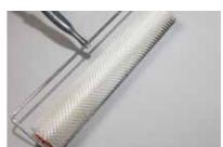
14. Immediately after smoothing the material should be de-aired with a spiked roller. Spiked shoes must be worn during application while walking over the fresh material.
