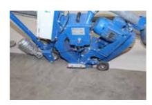
2. Floors and screeds must also be shot blasted to roughen the surface and produce an open pored, absorptive surface.
